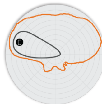
Figure 5. T750 5GHz Elevation Antenna Patterns
